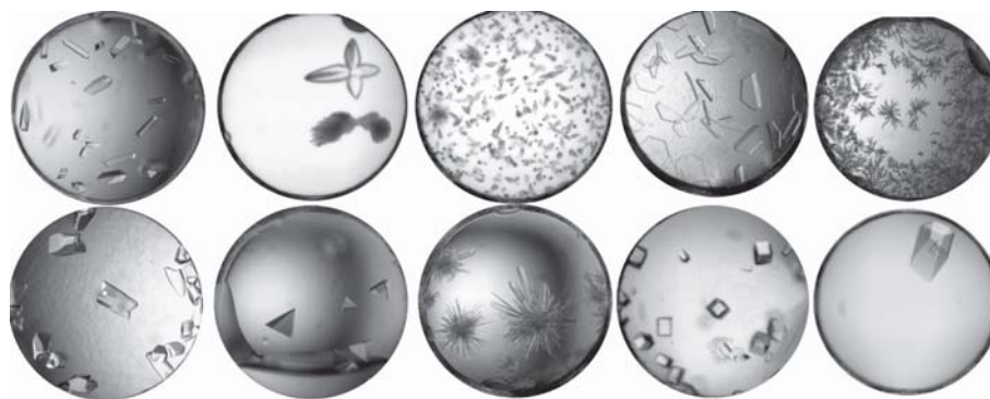
Figure 2. High-throughput microbatch-under-oil screening outcomes from our laboratory that show examples of crystal leads for several different proteins. Each image displays a well of 0.9 mm diameter. Some hits are obvious crystals, others need closer examination and are more difficult to discern on the scale of the figure.
