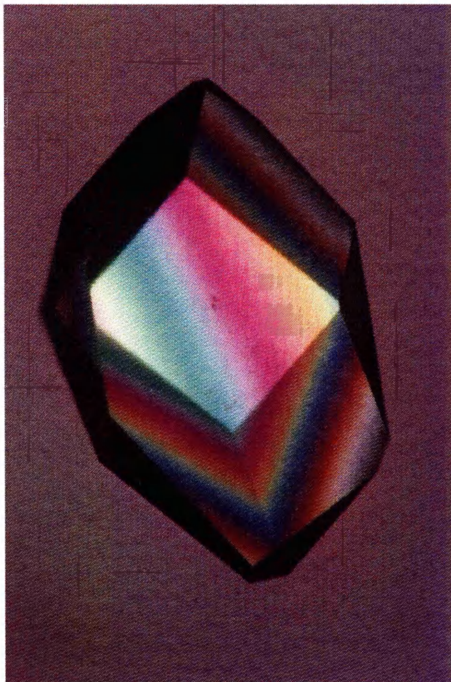
Figure 8.6: Photograph of typical tetragonal crystal produced on the IML-2 mission. Crystal length, along the longest dimension, 2.5 mm
