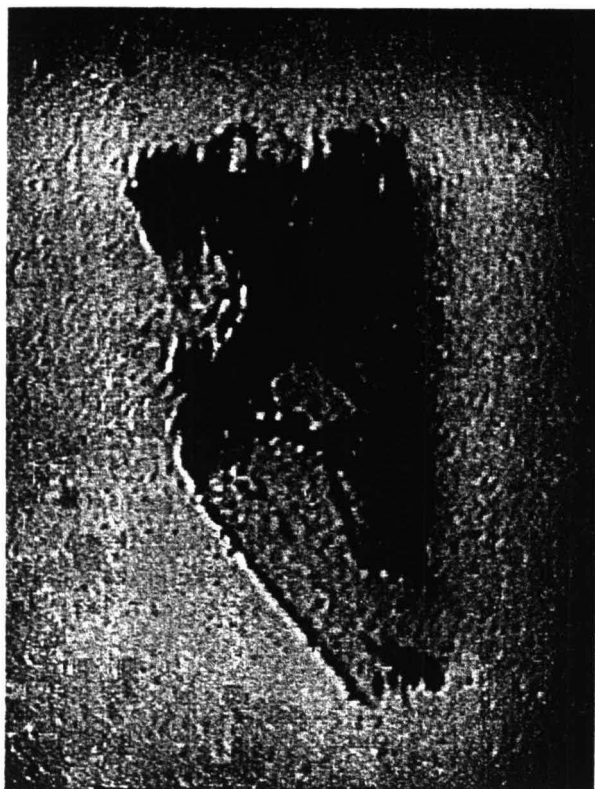
Fig. 8. X-ray topograph of a lysozyme crystal. (Based on Stojanoff et al. (1996)).
