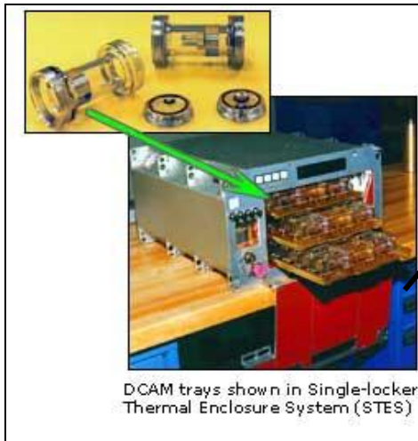
(c) DCAM - Diffusion-controlled Crystallization Apparatus for Microgravity
