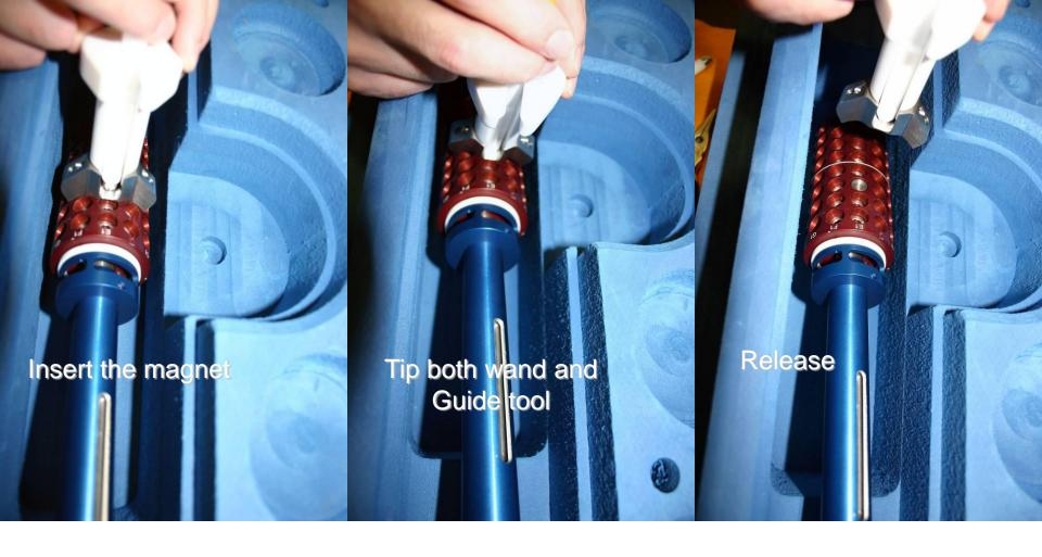
The magnet head can sticks to the wand due to ice between the two. To overcome this push the magnet in with the wand following the guide tool, then tip both the wand and guide tool together. The magnet will remain in the cassette. New tools with a push release can also develop the same problem (with a similar solution).
