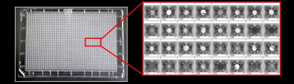
The crystallization method used is micro-batch under oil with 200 nl of protein solution being added to 200 nl of precipitant cocktail in each well of a 1536 well plate.
